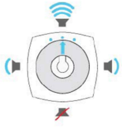
4. Close to the limit on the top. The speaker on the top increases its volume and the speaker on the side keep decreasing their own. plays Polar array of LEDs keep shrinking down.
