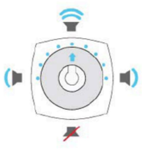
3. Keep pushing up. The speaker on the bottom is muted, the speakers on the sides start decreasing their volume level. LEDs keep turning off from the bottom-top.
